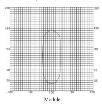
The arc region is the area where an  $\Phi$ 7.5cm round stick can be detected.
