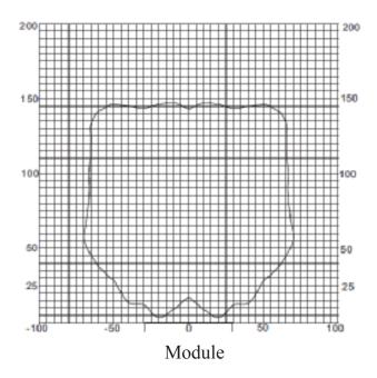
The arc region is the area where an  $\Phi$ 7.5cm round stick can be detected.
